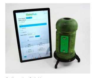
Online, the GaiaXus system connects to a secure AWS cloud where data is stored, shared, and mapped using the GIS standard tool, ArcGIS. Its open data architecture enables easy downloads of raw files and supports the development of offline lesson plans for community engagement and education.
